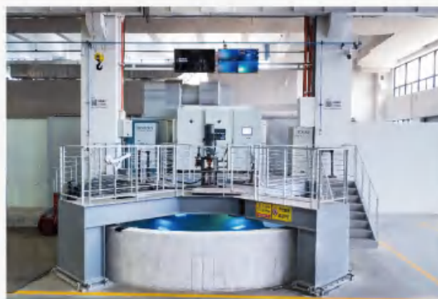
110方水试槽:5.4Mx5.2M
